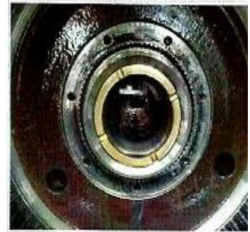
Sun gear Thrust Washer Damage
