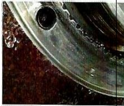
Spindle Retaining Nut Loose
