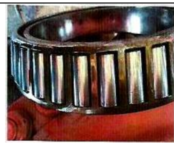
Bearing Cone Prior to remove of Cage
