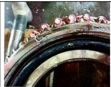
Brake Seal Installing Damage
